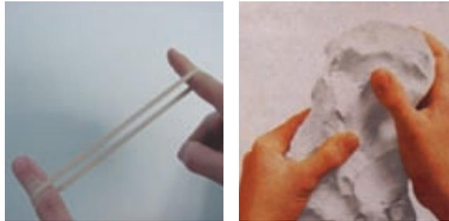
An example of a plastic polymer is the low molecular weight **polyisobutylene (PIB)** which is a synthetic polymer originating from the oil industry. This polymer shows a high degree of fluidity (or flow), meaning that, if left in a container, it will eventually flow over the bottom taking its exact shape. This property is exactly what is required for the adhesive to align itself with the skin surface, allowing it to make full contact with the skin.
